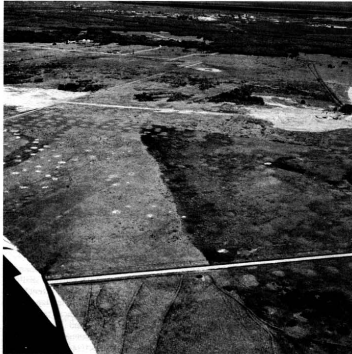
Figure 4. A copy of a color IR photograph taken at an altitude of about 300 m. The upthrown side of the fault is typically lighter in color. The more luxuriant vegetation, wet ground, and occasional sag ponds give the downthrown side a darker color. The apparent abrupt termination of the fault at the fence line is an illusion caused by a difference in land use. The scarp can be traced northeastward for another kilometer.
